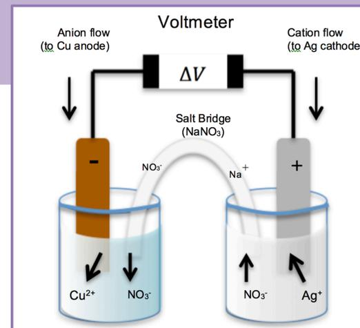
Figure 1. Representation of a typical  $Cu(s) | Cu(NO_3)_2 || Ag(NO_3) | Ag(s)$  galvanic cell.
