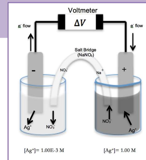
Figure 2. Representation of a Silver concentration cell.
