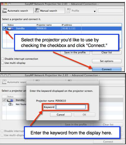
22. Check the Checkbox next to the projector you would like to use and click "Connect." Enter the keyword from the display, then use the control panel to control when you are sharing your screen.
